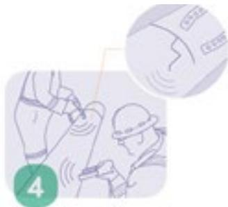
**4** Remove the coating, clean the pipe surface, and visually inspect any anomalies with magnetic particle inspection and ultrasonics. Divert the product around the segment that's being repaired.
